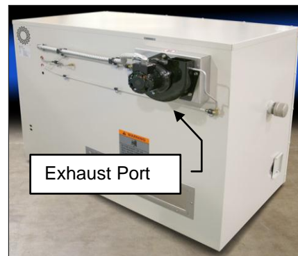
Figure 6. Exhaust Port on the Rear Right of the RFD1-42-2E Oven.
